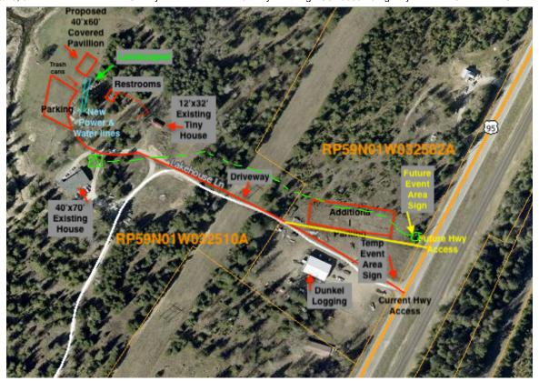
The depth of the cable must remain 36" or greater, any grading or excavation on the property must preserve the cable burial depth. The applicant is required to call 811 for utility locates prior to any dirt work.
